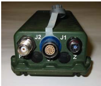
Figure 5. Communications Network Radio Sub-System (CNRS).
